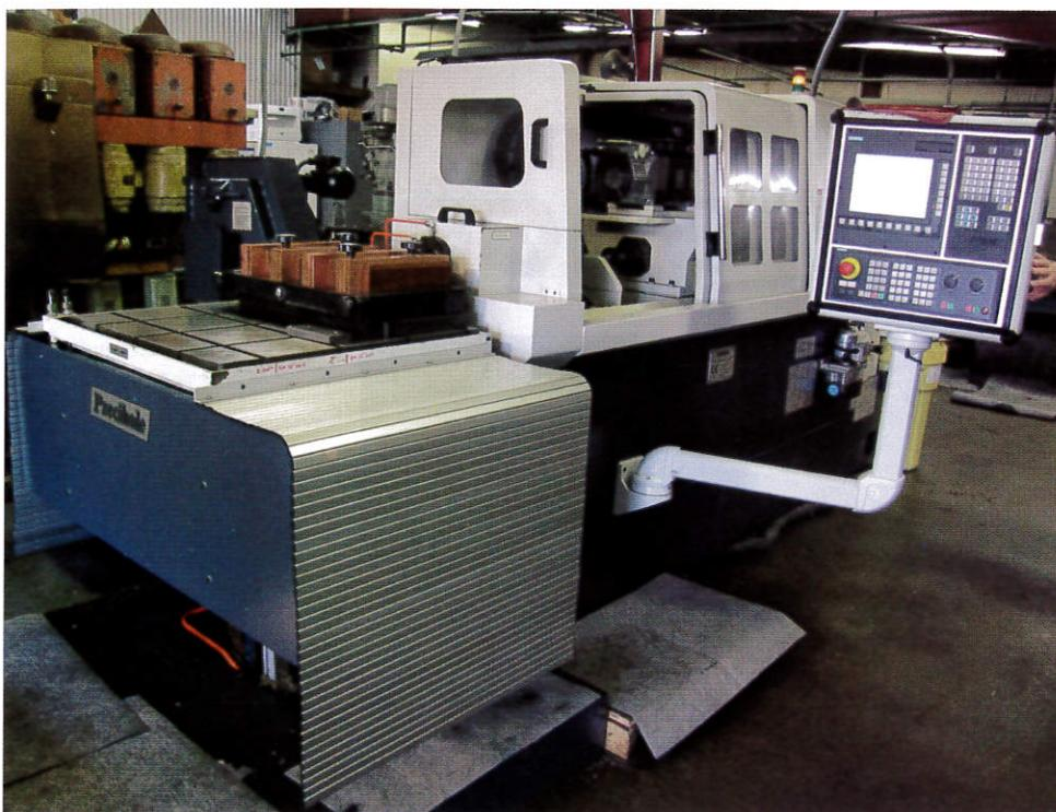
The company upgraded its deep-hole drilling capability with this three-axis machine from Precihole. The programmable X/Y table provides flexibility for multipart processing in a single setup. The table has 500 mm (19.7 inches) of cross travel in the X axis and 300 mm (11.8
