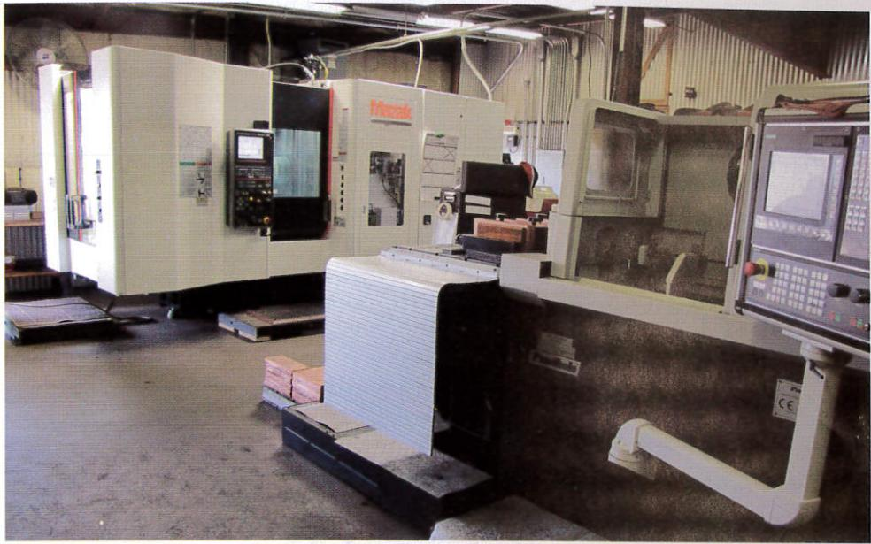
The deep-hole machine was installed next to an HMC equipped with a pallet changer. The two new machines can be used together as a single cell to produce the chill blocks.
